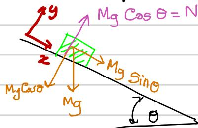
The only forces acting on the block are the gravitational force and the Normal force.
