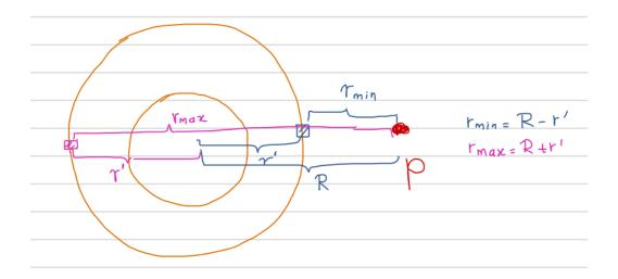
$r_{min} = R - r'$  and  $r_{max} = R + r'$
