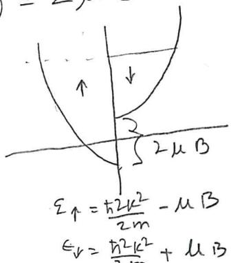
The split-band, therefore, merely reflects that energy of  $\uparrow$  moments have reduced by  $-\mu B$  for all electrons irrespective of  $k$  value, and energy of all  $\downarrow$  moments have increased by  $+\mu B$ . This picture carries over to the case of Ferromagnets.
