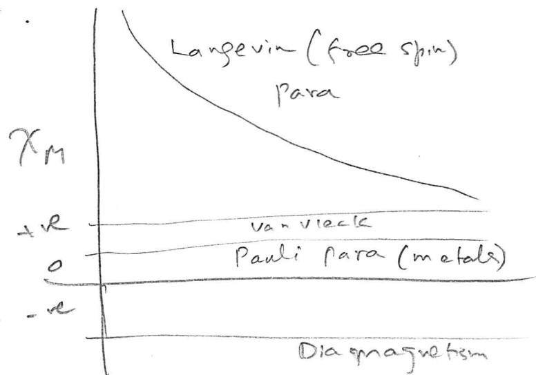
Most electrons cannot respond to external field because states are already occupied. Only electrons within  $k_B T$  can respond. Only a fraction  $T/T_F \approx 0.01$  contribute to spin susceptibility.
