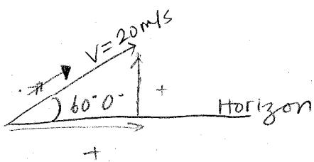
$$V_x = V_0 \cos \theta = (20 \text{ m/s}) \cos 60 = 10 \text{ m/s}$$
