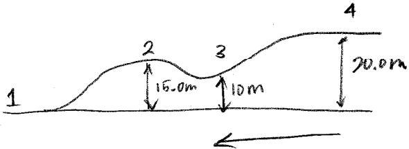
$$n=1 \quad v_1 = \sqrt{(12 \text{ m/s})^2 + 2(9.8 \frac{\text{m}}{\text{s}^2})(20 \text{ m} - 0 \text{ m})} = 23.2 \text{ m/s}$$
