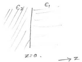
② Let us consider the case  $z' < a$ , which corresponds to finding the electric potential due to a unit point charge inside the dielectric material  $\epsilon_2$ .
