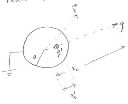
② Electric field is zero inside a conductor, and can have only components normal to the surface. Any constant electric potential will achieve this. A grounded conductor means that this constant is chosen to be zero. Thus, we have.
