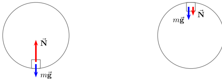
Figure 7.8: Forces acting on a mass while moving in a vertical circle inside a globe.
